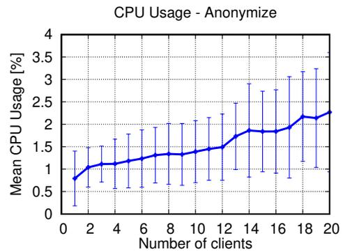
**Fig. B.7.** CPU usage on the relay during Anonymize, averaged over 10 minutes. The client are real Android and iOS devices (hence the x axis stopping at 20). The relay’s hardware is a commodity server with a 3GHz Xeon Dual Core and 2GB of RAM. If we extrapolate the linear tendency, we estimate the mean CPU usage to be below 10% with 100 clients in this setup.
