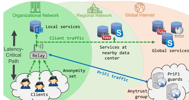
**Fig. 1.** PriFi’s architecture consisting of clients, a relay, and a group of anytrust servers called the *guards*. Clients’ packets remain on their usual network path without additional hops, unlike in mix-networks and onion-routing protocols.
